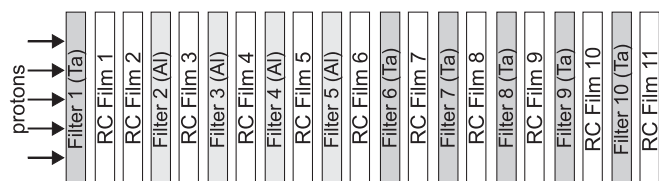
FIG. 8. Radiochromic (RC) film pack design for detection of proton radiographs. The pack consists of interleaved filters (Al or Ta) and films.
